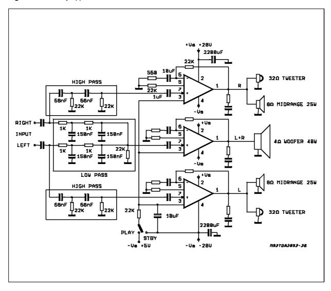
As shown in Figure 19, the R-C passive network for low-pass and High-pass give a cut with a slope of 12dB/octave
