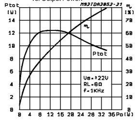
**Figure 12:** Total Power Dissipation & Efficiency vs. Output Power.
