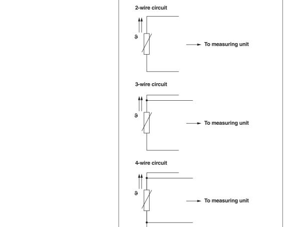
Figure 4: Methods of connection
