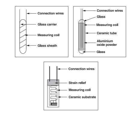
To protect them against mechanical damage (pressure or flowing liquid) these measuring elements are usually installed into suitable protective tubes (measuring inserts). This also ensures easy replacement without the need to replace the complete fitting. As resistance thermometers are contact-making temperature sensors (i.e. the sensor has to reach the temperature of the medium in which measurement is to be performed) the housing has to be adapted to the application (see Fig. 3).
