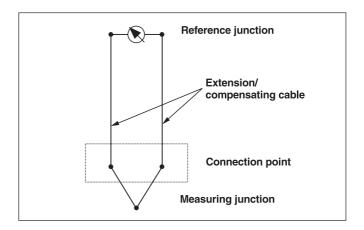
The thermoelectric voltage appearing at the reference junction depends on the thermocouple wire material and on the temperature difference between the measuring junction and the reference junction. For temperature measurement, the temperature of the reference junction must be kept constant (e.g. 0 °C) or must be well known, to make a appriopriate correction in mV (see Fig. 6).
