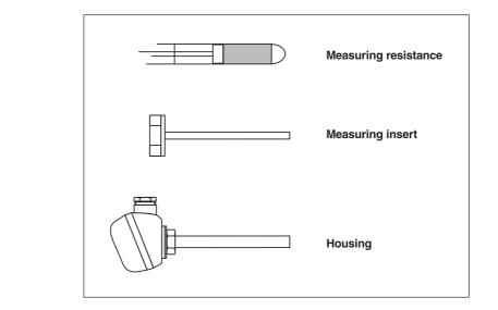
Figure 3: Resistance thermometer modules
