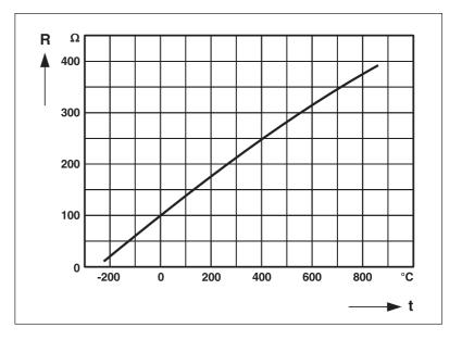
Figure 1: Pt 100 characteristic curve
