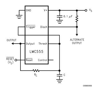
FIGURE 12. 50% Duty Cycle Oscillator
