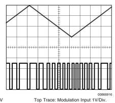
FIGURE 11. Pulse Position Modulator Waveforms
