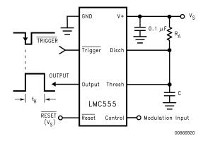
FIGURE 8. Pulse Width Modulator
