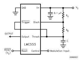
FIGURE 10. Pulse Position Modulator
