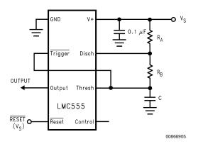
FIGURE 4. Astable (Variable Duty Cycle Oscillator)
